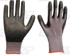
PT-N101S-2 Liner:15G nylon Coating:nitrile foam with nitrile dots Size:7-11 CE EN388:4121X
