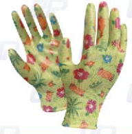
PT-N101P Liner:13G polyester/nylon Coating:nitrile smooth Size:7-11 CE EN388:4121X
